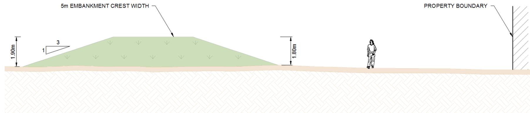
**Section A-A: Indicative Embankment Cross Section**
