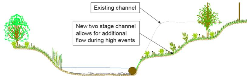
Typical example of a two stage channel
